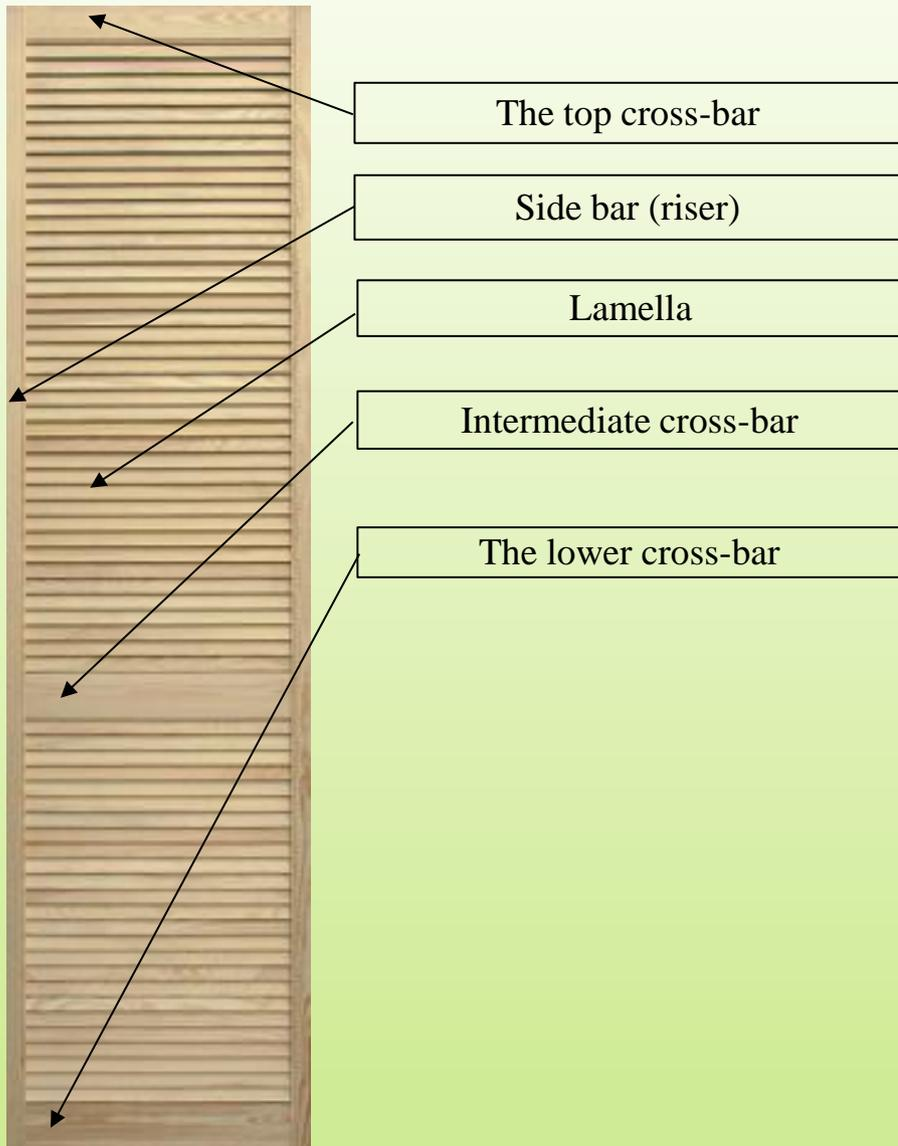
Side bar (riser) is produced by grafting technique, which prevents longitudinal deformation. Cross-bars are fixed to the side bars by means of dowels.
